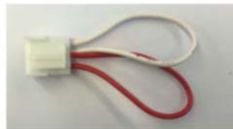
Figure 2: connector with short-circuited wirings
